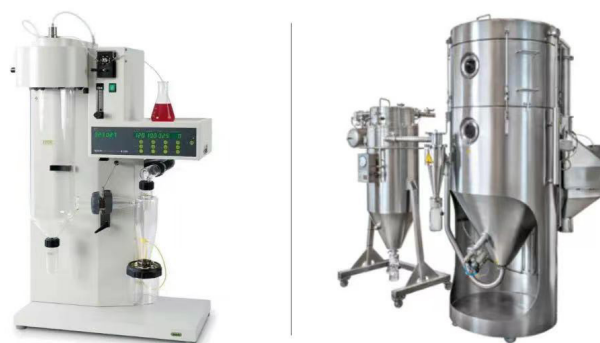
Figure 2. Spray Drying Equipment Utilized at Crystal Pharmatech (Buchi B-290; GEA PSD-1)
